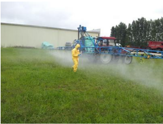
Figure 8: Boom section test, pressure homogeneity test, pressure drop test. Source GIPPulves
