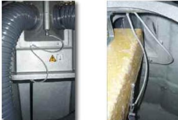
Fig. 7 – Example of static discharge devices (Photo: Spanish manual for the inspection of the sprayers in use)
