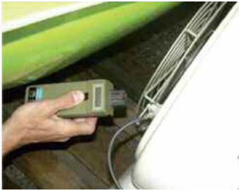
Fig. 18 - Check of the fan rotational speed with the tachymeter (optional)
