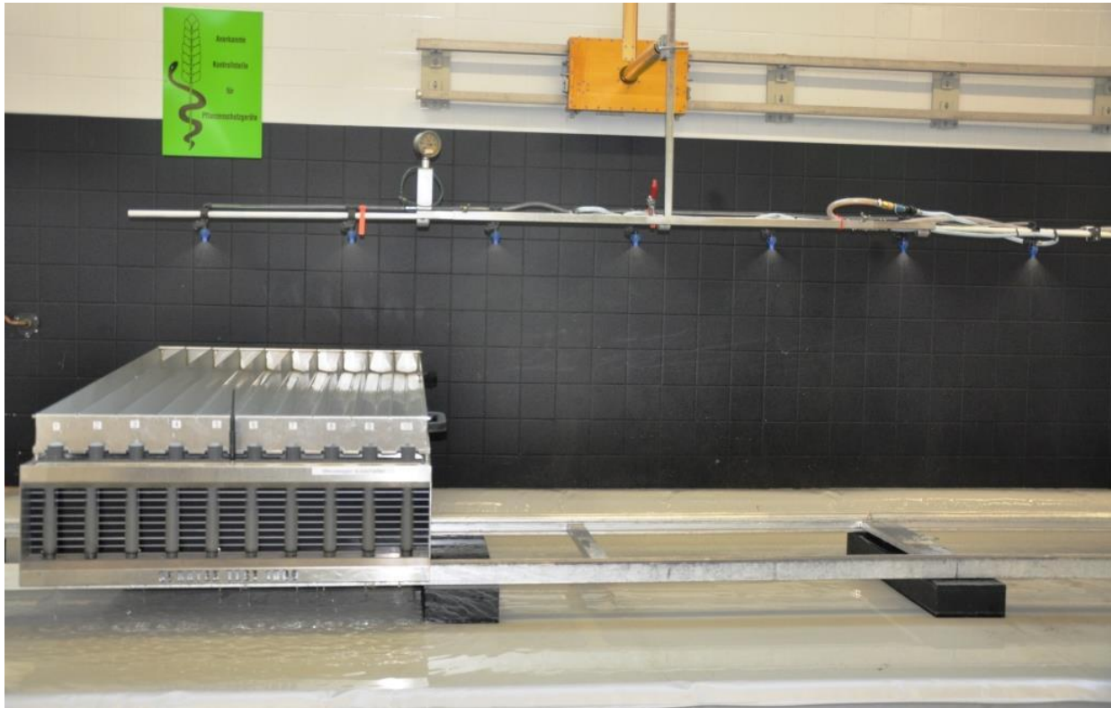
Picture 1: plot spray boom patternator test system used at Bayer AG
