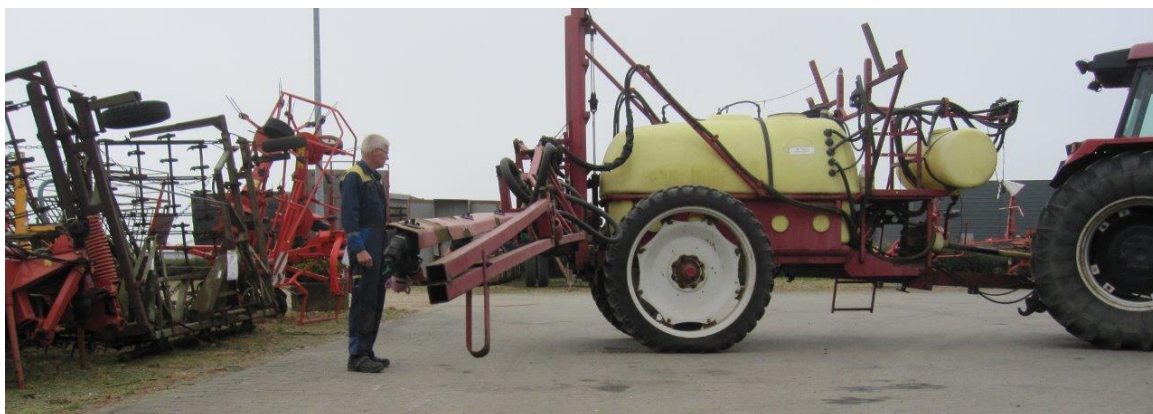
Photo 1: Boom stability, as well as nozzle orientation are defects often found on older sprayers.
