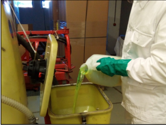
Figure 28: Induction hopper without CTS
