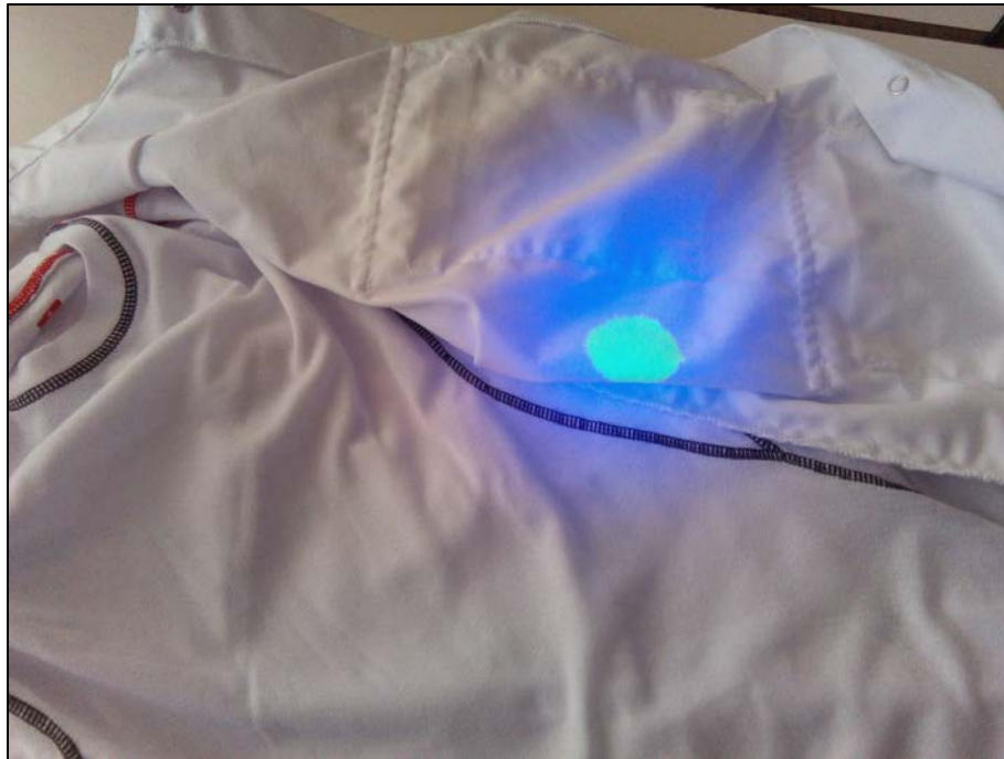
Figure 14: In the case of contamination of the overall jacket, no tracer is absorbed by the underlying polyester underwear, and instead the drop only spreads within the jacket fabric
