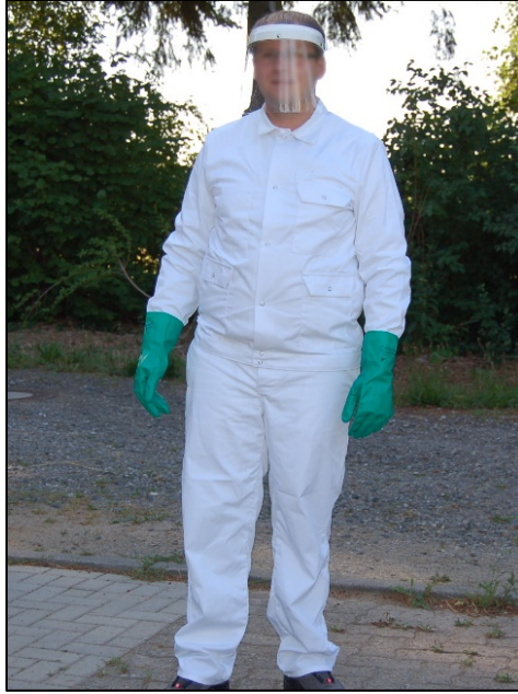
Figure 18: Outer dosimeters (protective overall, protective gloves and protective visor)
