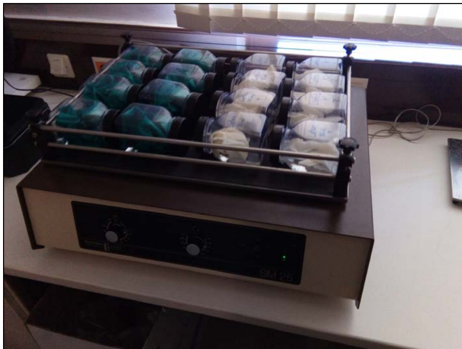
Figure 16: Protective gloves and laboratory gloves in PET containers on the laboratory shaker
