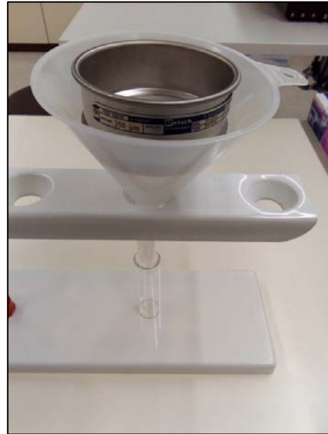
Figure 11: Setup for filtration with stainless steel sieve (250 \mu\text{m} mesh size)
