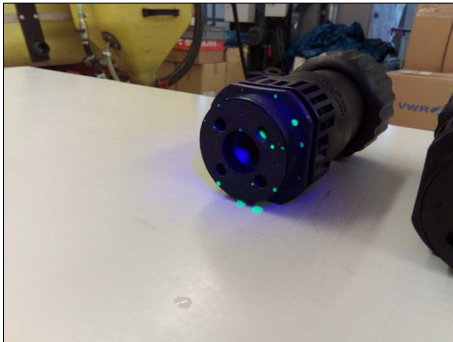
Figure 34: Contact surfaces of the canister adapter after the filling cycle
