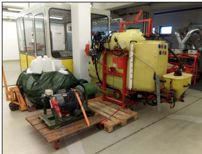
Figure 22: Experimental setup of the field crop sprayer with drive motor
