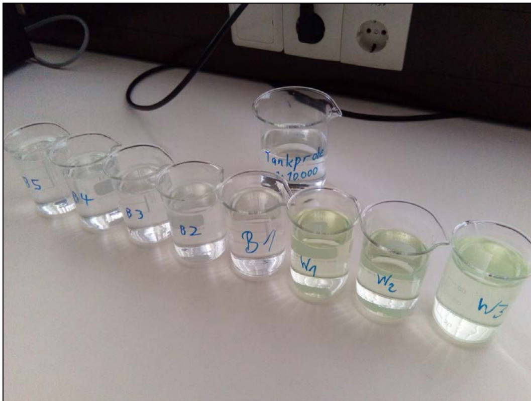
Figure 15: Green color of the water in the recovery experiment (three glasses on the right) compared to the blanks (on the left) and for dilution with the same concentration (large glass in the background)
