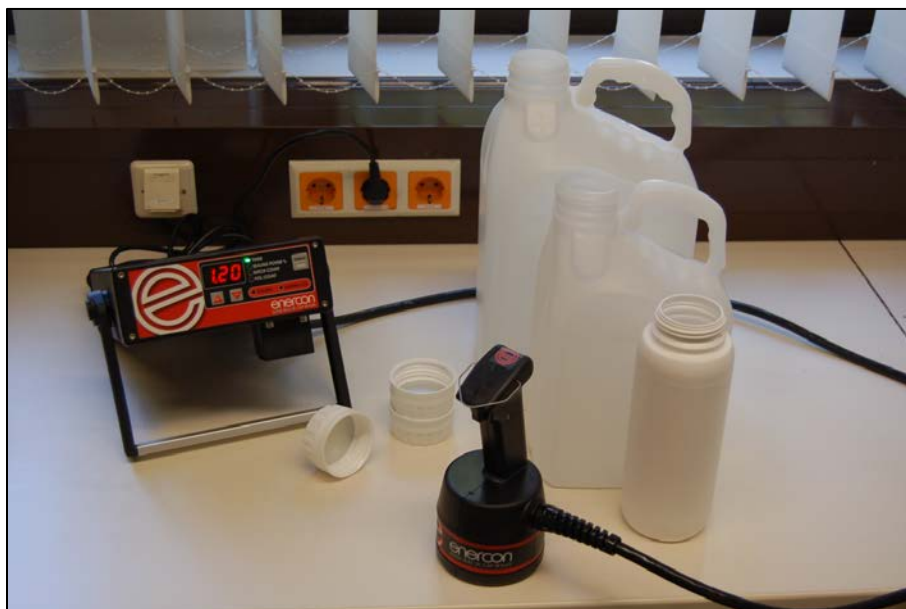
Figure 24: Sealing device with canisters and caps
