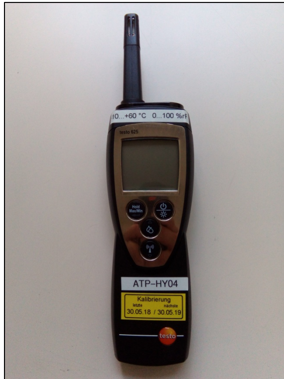
Figure 26: Hand-held meter (testo 625) for measuring temperature and humidity
