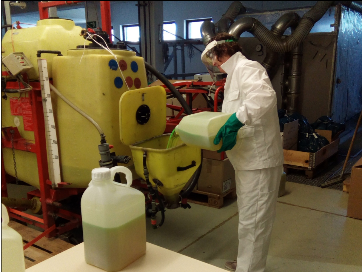
Figure 27: Carrying out a filling test at the induction hopper without CTS
