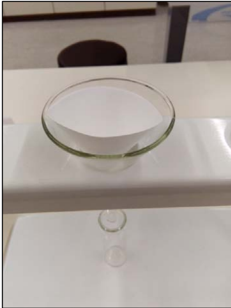
Figure 10: Setup for filtration with filter paper
