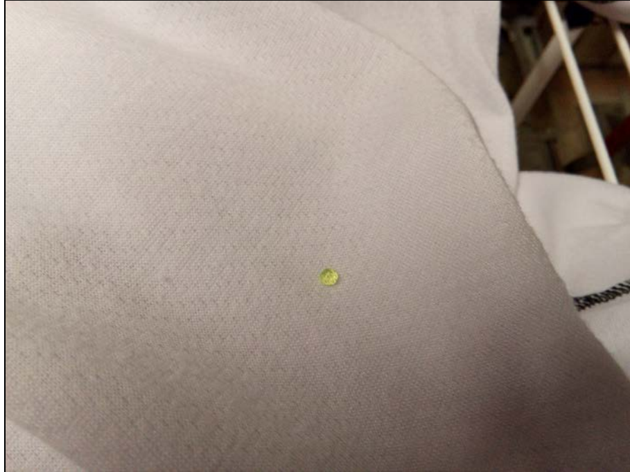
Figure 13: Drop of the tracer, which rests outside of the polyester fabric and rolls off
