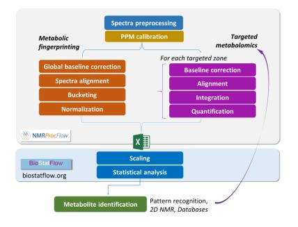
For Metabolic Fingerprinting or Targeted Metabolomics, NMRProcFlow workflow covers all steps from spectral data to data matrix
