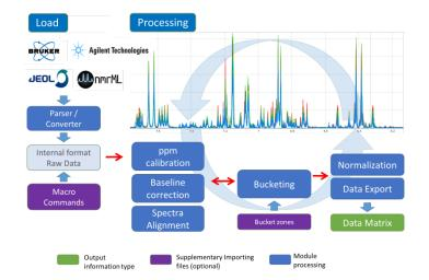
NMRProcFlow covers all spectra processing steps including baseline correction, chemical shift calibration and alignment
