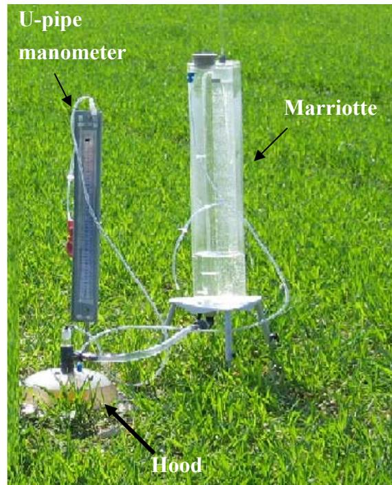
Photo. 8: Infiltration measurement using a Hood Infiltrometer
