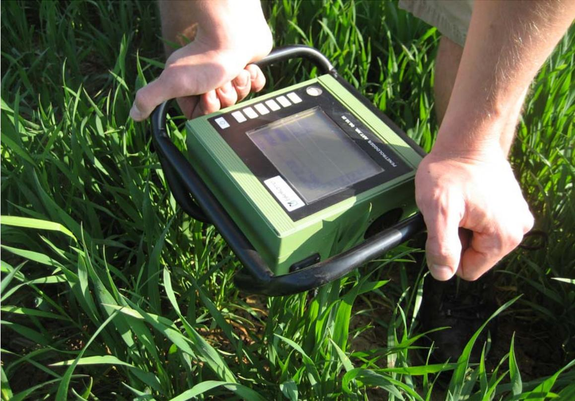
Photo. 7: Measurement of soil penetration resistance using a Penetrologger
