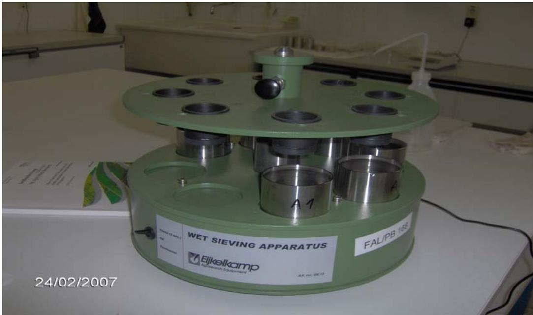
Photo. 5: Soil aggregate stability determination using a wet sieving apparatus
