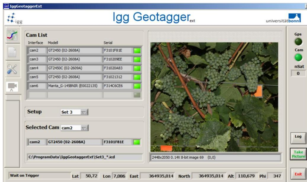
**Figure 1.** Graphical user interface of the *IggGeotagger.Ext*. The software manages the communication between the control unit of the *PHENObot* and the image acquisition PC, triggers the cameras and controls the image transport and storage. It is preferentially used for the visualization of captured images and for setting the camera parameters.
