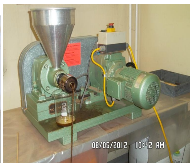
Figure 2.5: Extraction of neem oil using mechanical press
