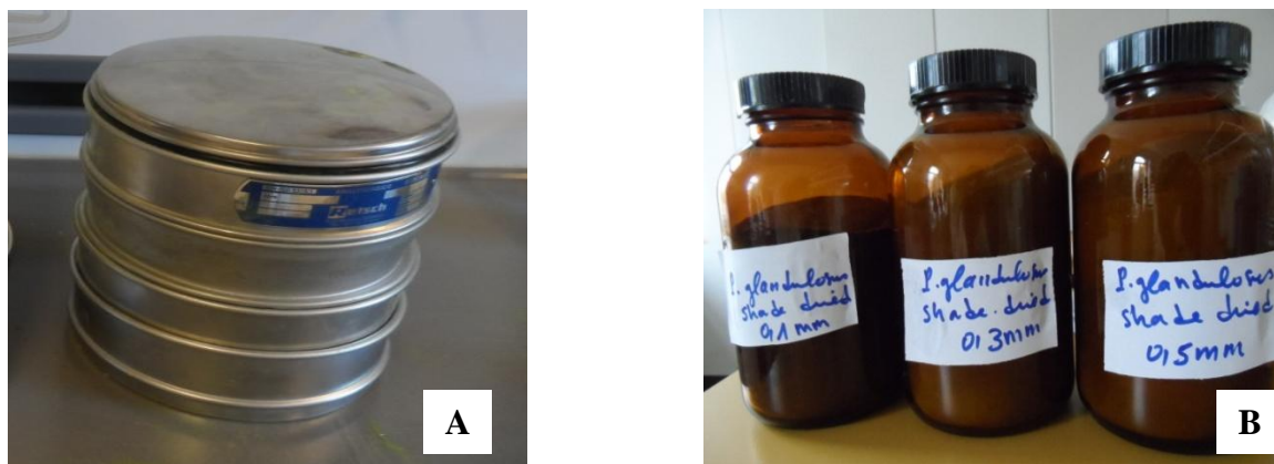
Figure 2.7: The three analytical sieves used to obtain different particle size powders (A) and glass jars containing the leaf powders of different particles sizes ( \leq 0.1 mm, \leq 0.3 mm, \leq 0.5 mm) (B)
