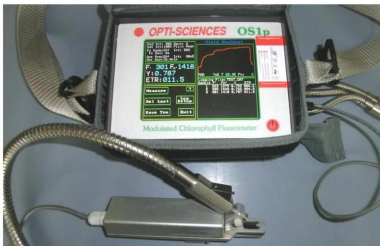
**Figure 5. OS1p-Chlorophyll fluorometer.** The display shows three exemplary measurements down right and general settings top left. Besides this, the leaf clip for measurement is shown consisting out of the clip with the trigger button and the sensor for detecting the photosynthetic active radiation (PAR).
