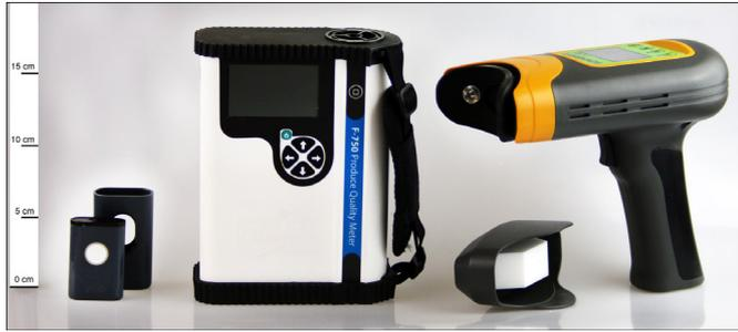
**Fig. 1:** Commercially available portable NIR food-scanner: (left) SCiO™ Molecular Sensor with protective plastic case, (middle) F-750 Produce Quality Meter, (right) H-100F portable spectrometer with protective plastic cap.
