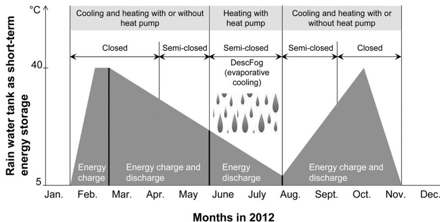
**Fig. 1:** Schematic diagram for closed and semi-closed operation phases in the confined closed greenhouse system and associated energy charge and discharge processes occurring in the short-term energy storage tank.
