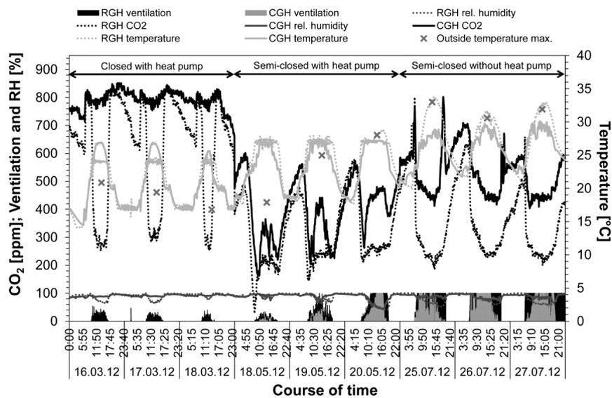
**Fig. 2:** Comparisons of microclimatic conditions and the ventilation behaviour between the reference greenhouse (RGH) and the confined closed greenhouse (CGH) in consideration of selected days during winter, spring and summer.
