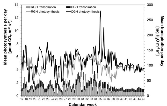
**Fig. 3:** The mean daily photosynthesis (GECO<sub>2</sub>) and plant transpiration caused by the reference greenhouse (RGH) and the confined closed greenhouse (CGH) during harvest time.
