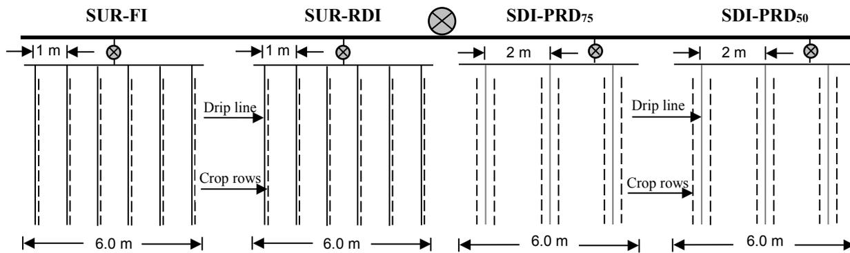
**Fig. 1:** Layout of the experimental plots showing drip line positions and arrangement of tomato plants under different drip irrigation treatments. FI = full irrigation; PRD = partial root zone drying; RDI = regulate deficit irrigation; SDI = subsurface drip irrigation; SUR = surface drip irrigation.
