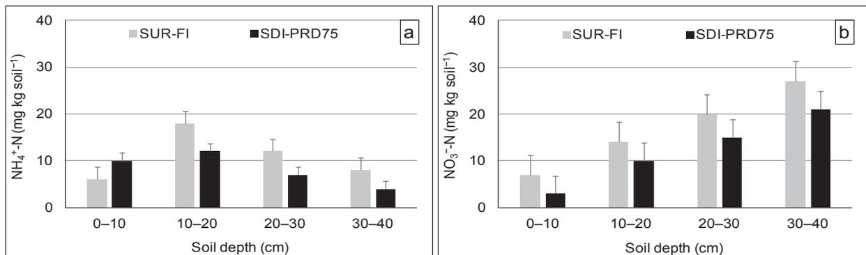
**Fig. 5:** Soil residual  $\text{NH}_4^+$ -N (a) and  $\text{NO}_3^-$ -N (b) contents at different soil depths for SUR with FI and SDI with (PRD<sub>75</sub>) at the last harvest of tomato in 2016. Error bars indicate standard error of the means ( $n = 3$ )  $\pm$  S.E.
