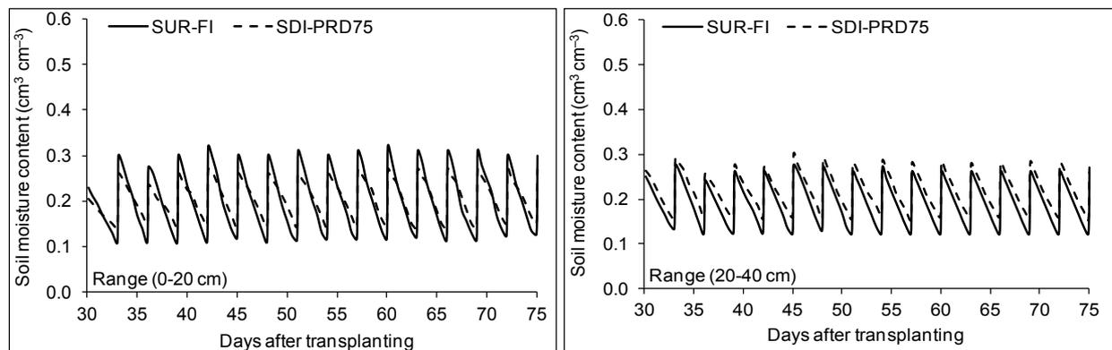
**Fig. 2:** Temporal changes of moisture content in two different soil layers during the developmental stage for SUR with FI and SDI with PRD<sub>75</sub> (pooled data of the two years).
