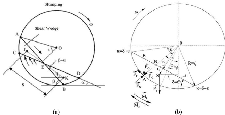
**Fig. 2:** (a) Material bed motion in slumping mode, and (b) material bed motion in rolling mode.
