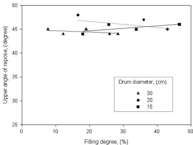
**Fig. 5:** Effect of filling degree on upper angle of repose for cylinders with diameters equal to 15, 20, and 30 cm.
