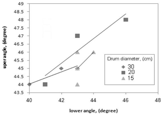
**Fig. 6:** The differences between lower and upper angles of repose in rice grains due to different filling degrees and cylinder diameters ranges from 1° to 4°.
