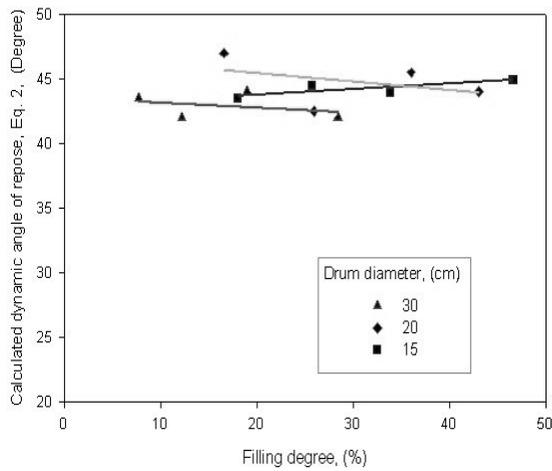
**Fig. 7:** Effects of filling degree on calculated dynamic angle of repose using Eq. (5) for cylinders with diameters equal to 15, 20, and 30 cm.
