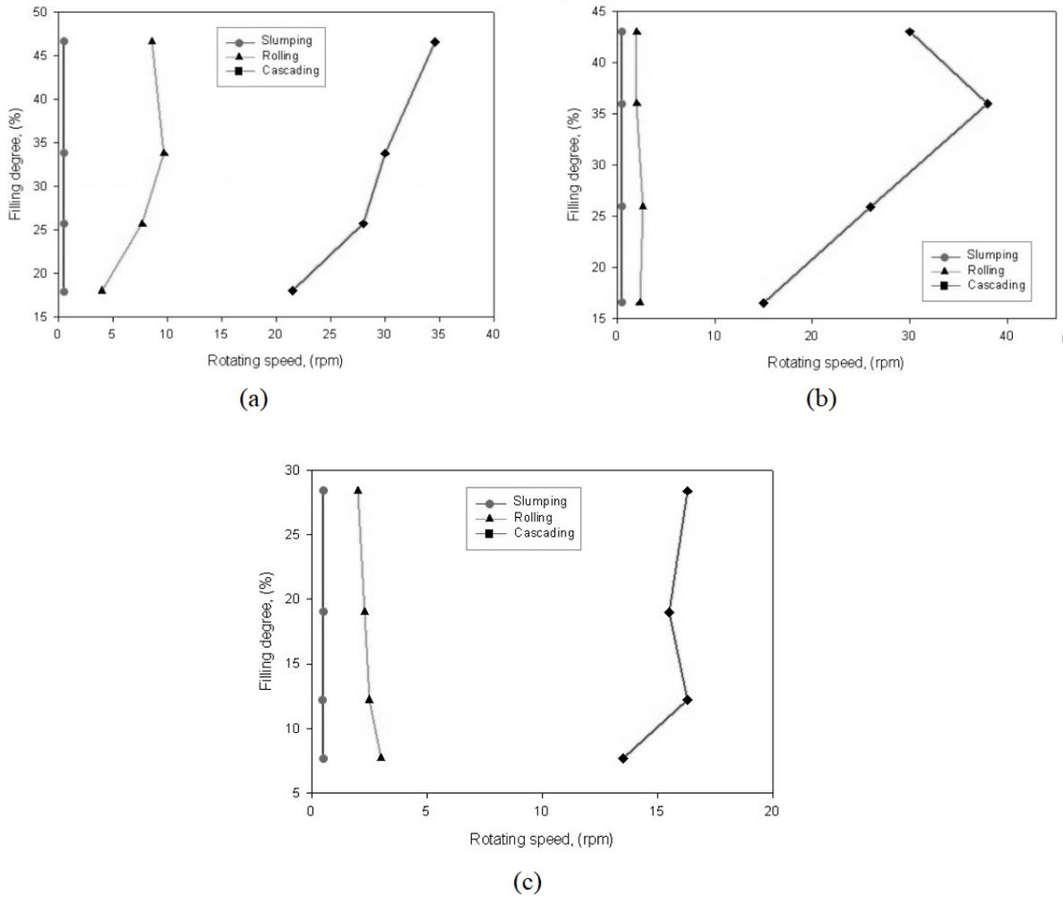
**Fig. 4:** Filling degree at different rotating speeds in slumping, rolling, and cascading modes for cylinders with diameters equal to (a) 15 cm, (b) 20 cm, and (c) 30 cm.
