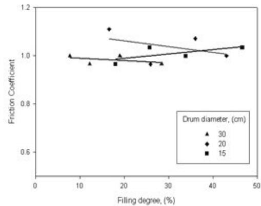
**Fig. 8:** Effects of filling degree on friction coefficient of rice grains for cylinders with diameters equal to 15, 20, and 30 cm.
