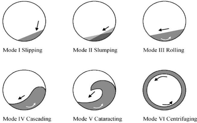
**Fig. 1:** Transverse motion modes of materials in a rotating cylinder (KHAZAEI and GHANBARI, 2010).
