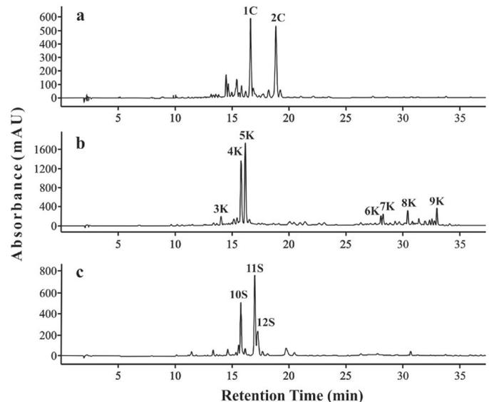
**Fig. 2:** Comparative HPLC-DAD chromatograms at 320 nm of phenolic profiles in *Echeveria* species. (a) *E. craigiana*, (b) *E. kinnachii* and (c) *E. subrigida*. The tentative identification of the constituents is shown in Tab. 2.
