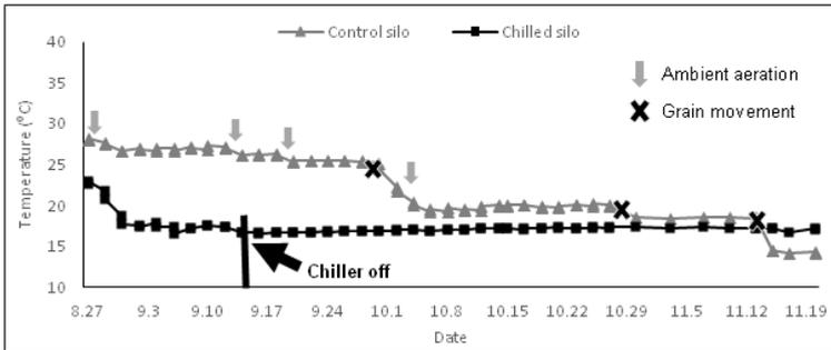
**Figure 8.** Grain temperature profile (°C) of the grain mass inside the Control and Chilled silo from Aug. 27<sup>th</sup> to Nov. 20<sup>th</sup>, 2015 in Farmer’s Cooperative, Kansas, U.S.A.
