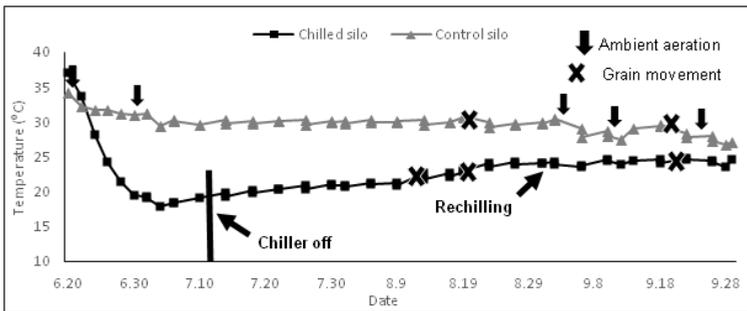
**Figure 9.** Grain temperature profile (°C) of the grain mass inside the Control and Chilled silo from June 20<sup>th</sup> to Sep. 29<sup>th</sup>, 2016 in Farmer’s Cooperative, Kansas, U.S.A.
