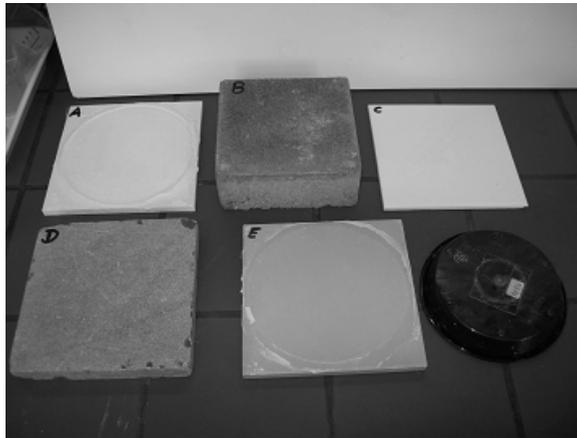
**Figure 1** Surface materials studied, (A) plywood, (B) concrete flagstone, (C) glazed ceramic flagging, (D) natural flagstone, and (E) porcelain stoneware, right to (E) plastic top for caging the insects.
