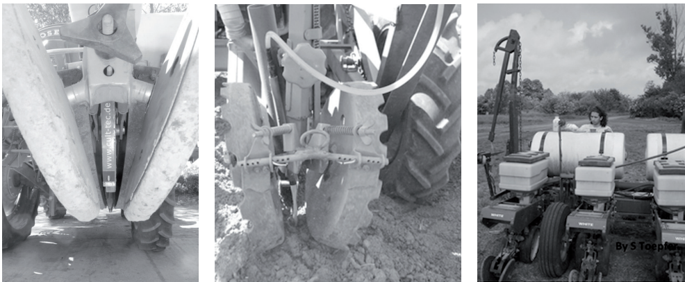
Fig. 2 Currently most promising and most used application technique for entomopathogenic nematodes against D. virgifera virgifera larvae: fluid stream spray application into the soil at sowing using sowing machines with applicators that apply nematodes behind the sowing wheel and prior the soil-closing wheels. Examples from left to right: LIQ-Inject M1 (Cult-tec company, Germany) on a Monosem NG Plus sowing machine (USA); Self-made application tube for fluids on Pneumasem sowing machine of Nodet Gugis( France); John Deere with fluid applicator on White sowing machine (USA).
