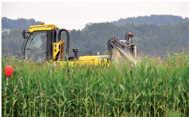
**Fig. 1** Specialized sprayer for tall crops during the drift measurements.
