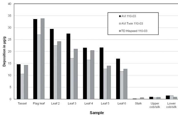
Fig. 3 Influence of nozzle type on spray deposition.
