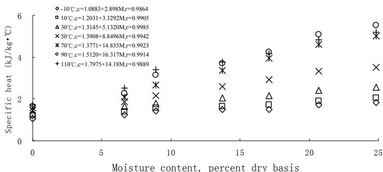
**Figure 4** Relationship between the specific heat and moisture content
