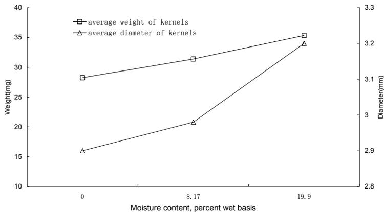
**Figure 5** Relationship among moisture content and weight, diameter of kernels
