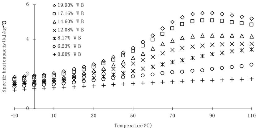
Figure 3 Relationship between the specific heat and temperature
