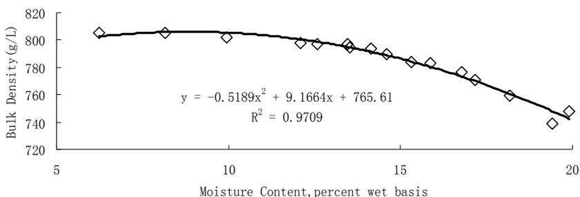
**Figure 1** Relationship between moisture content and the density of the wheat bulk.
