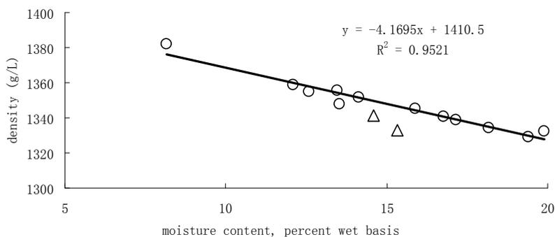
**Figure 2** Relationship between moisture content and the density of wheat kernels
