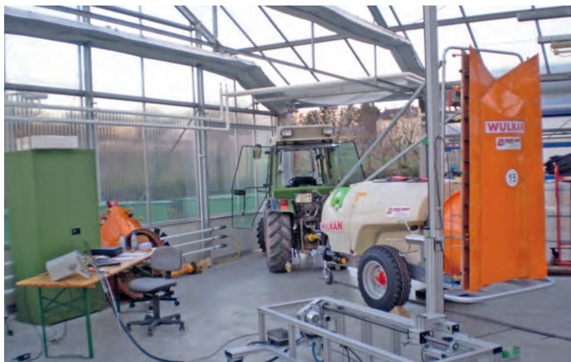
Fig. 1. View of air flow characteristic measurement unit based on isosonic anemometer.
