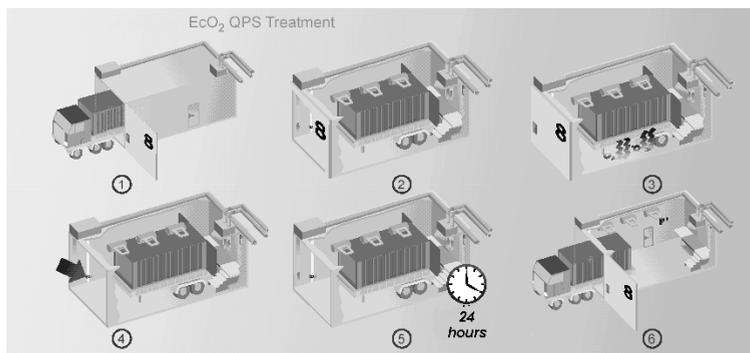
**Fig. 2** Schematic of the "EcO2 QPS Treatment" that complies with the ISPM 15 norm (EcO2, 2004)
