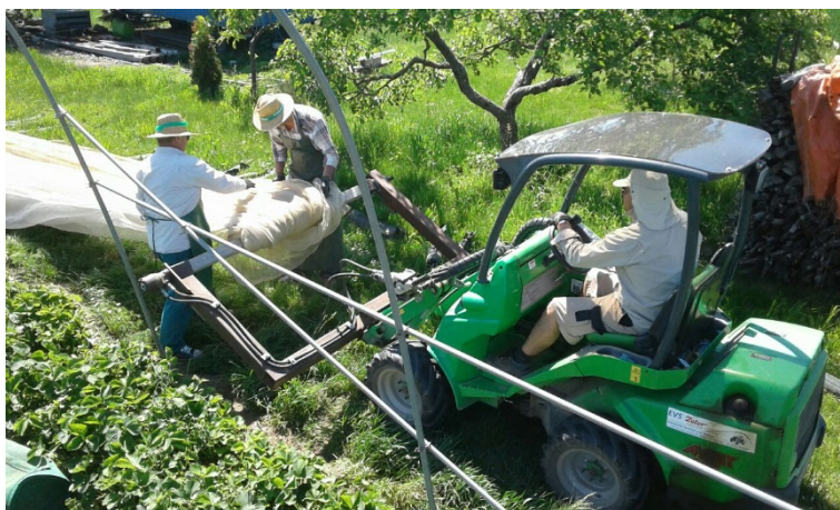
Photo 1 Furling of gauze, 20m /40m long, 3 times faster and more comfortable than by hand
