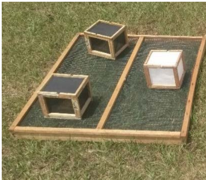
Fig. 3 Experimental cages for thermal disinfestation trials.
