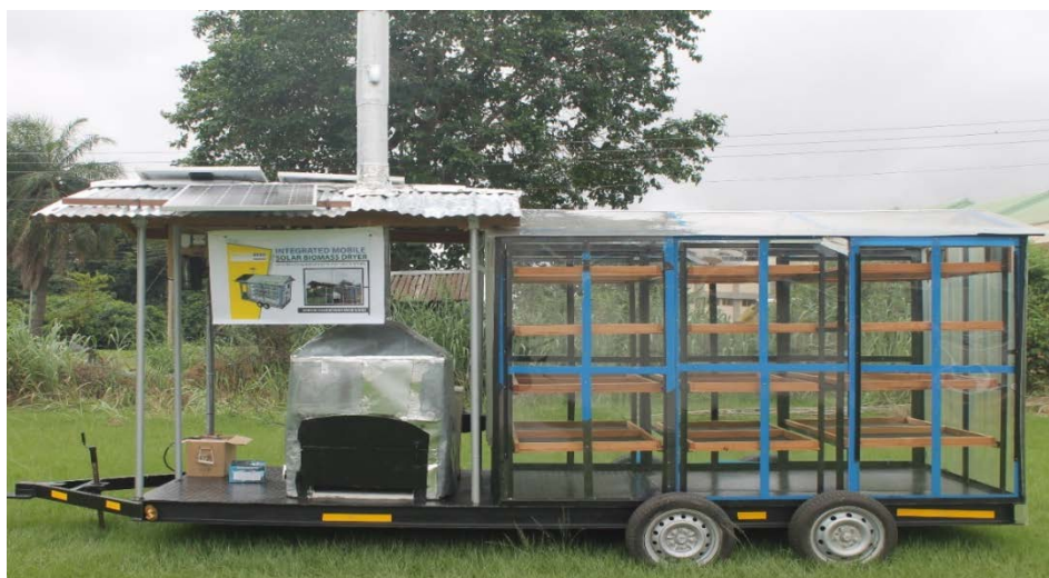
Fig. 1 Developed mobile solar biomass hybrid dryer at KNUST, Kumasi, Ghana.
