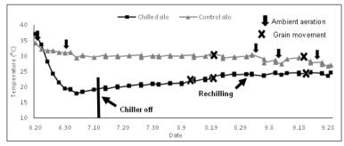
**Figure 9.** Grain temperature profile (°C) of the grain mass inside the Control and Chilled silo from June 20<sup>th</sup> to Sep. 29<sup>th</sup>, 2016 in Farmer's Cooperative, Kansas, U.S.A.
