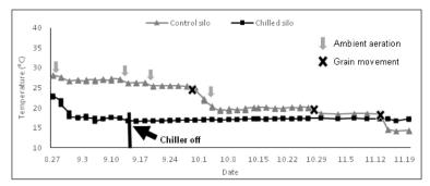
**Figure 8.** Grain temperature profile ( $^{\circ}$ C) of the grain mass inside the Control and Chilled silo from Aug. 27<sup>th</sup> to Nov. 20<sup>th</sup>, 2015 in Farmer's Cooperative, Kansas, U.S.A.
