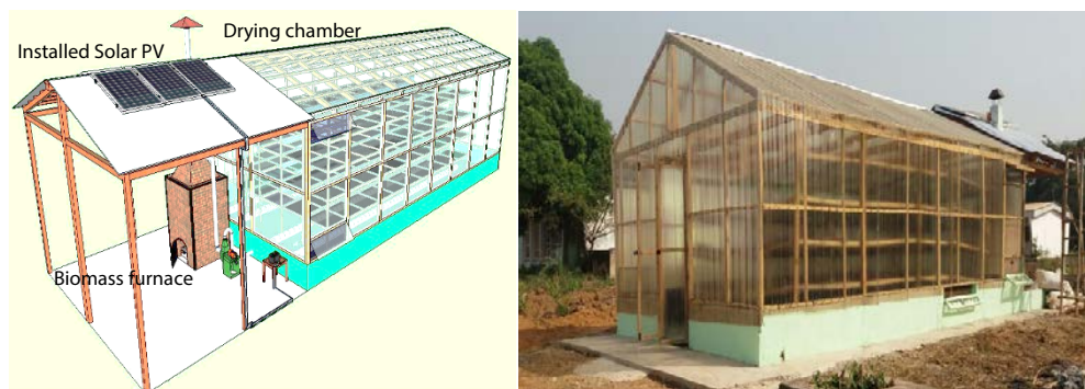
Fig. 1: Solar Biomass Hybrid Dryer; schematic view (left) and constructed view (right)
