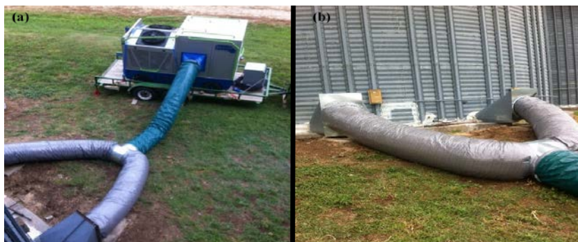
Figure 7. Grain chiller GCH-20 setup: (a) Insulated duct connected to the chiller's outlet at one end and to a "T" connector at the other, (b) Two ducts attached to the fan transition parts of the aeration fans that were removed.
