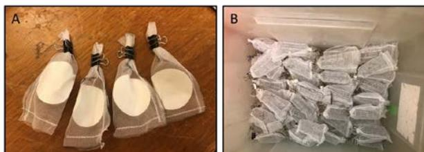
**Fig. 2** Nylon mesh cages containing fiberglass filter paper (A) and containing ACP (B). Note that the open end of the nylon cage was closed using a binder clip.
