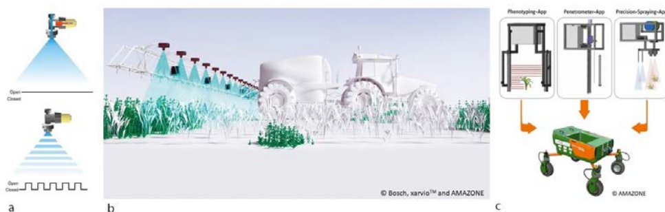
Fig. 1 Exemplary precision spraying systems – pulse width modulation (a), patch spraying of the SmartSprayer joint project (b), Bonirobot (c)
