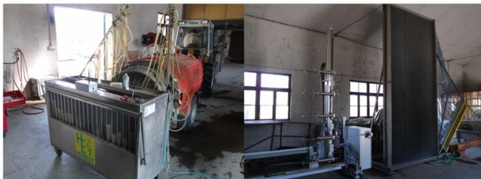
Fig 1. Test bench for the measurement of the flow rate of each nozzle (left) and of the liquid distribution (right).
