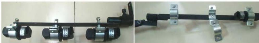
Fig. 2. Telescopic support for the flow meters enabling to measure liquid flows at different levels and from different directions.
