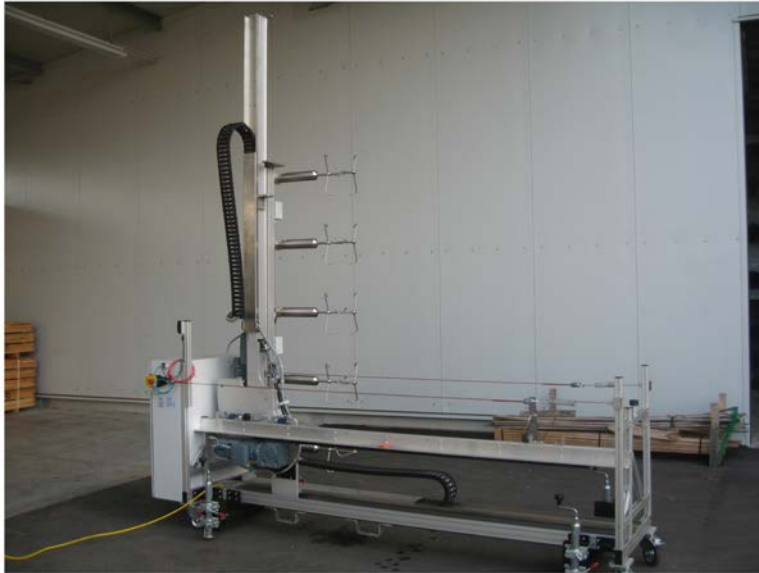
Fig. 5. The new air distribution test bench “WP 5000” (Photo: Triloff, 2012).
