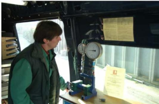
Fig. 5. Testing the sprayer manometer.
