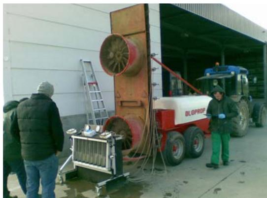
Fig. 1. Measuring nozzle flow rate and spray pressures.
