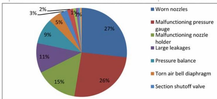
Fig. 4. An overview of category I defects during 2008-2009-2010 (Orchards sprayers).
