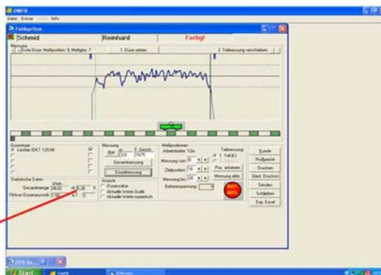
Graph 2. Cross distribution of IDKT 120-04C nozzles in use in combination with 4 x IDKN 120-04 in the mid section of the boom. Tested on Herbst scanner patternator SPRAYERTEST 1000
