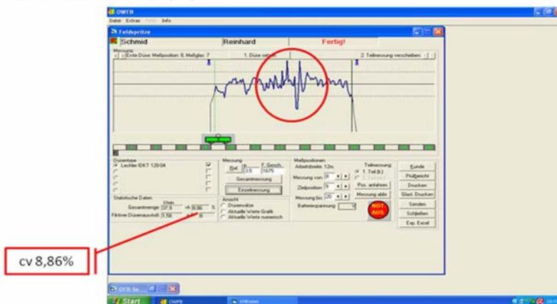
Graph 1. Cross distribution of IDKT 120-04C nozzles in use. Tested on Herbst scanner patterator SPRAYERTEST 1000
