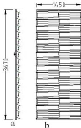
Fig. 14. The droplets intercepting patternator: a.lateral view; b. front view (dimension in mm).
