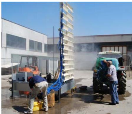
Fig. 4. The droplets intercepting patterator under test.
