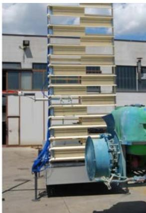
Fig. 5. Evaluation of the air velocity near the patterator.
