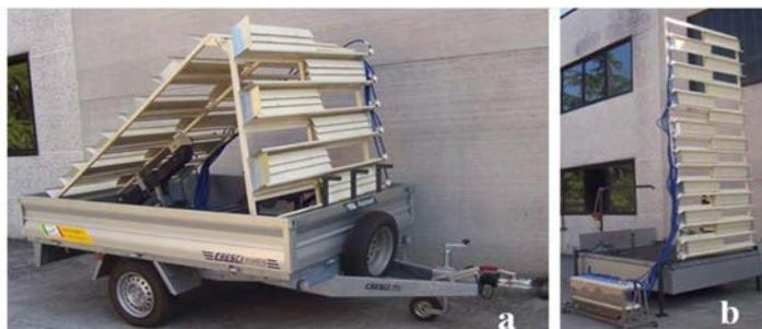
Fig. 2. The droplets intercepting patternator: a. folded on the bottom of the trailer; b. placed vertically.
