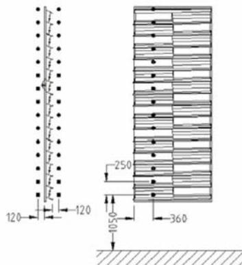
Fig. 6. Measure points of the air velocity (dimension in mm).
