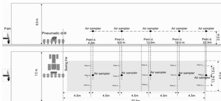
Fig. 1. The layout of CRA-ING testing area for checking pneumatic drills.
