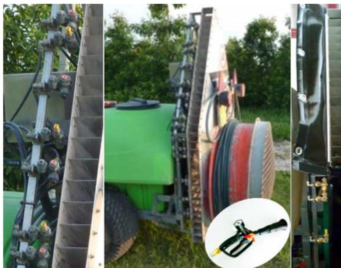
Fig. 15. Equipments compared during the test: particular of the side flow exclusion device (right), the double crown of nozzles (left) activated independently and the handheld gun fitted with manometer (oval box).
