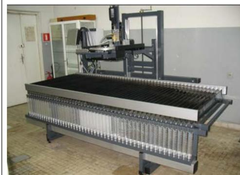
Fig. 3. Device to complex measurements of agricultural nozzles
