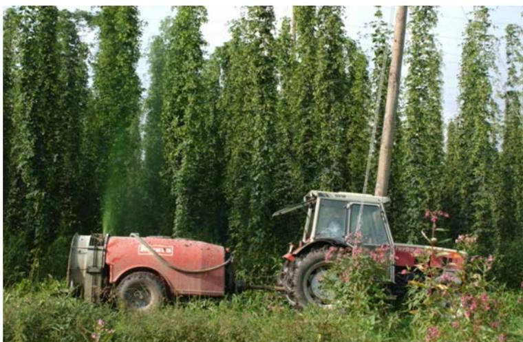
Fig. 4. Sprayer in hops with air injection nozzles and with shield on the fan outlet.
