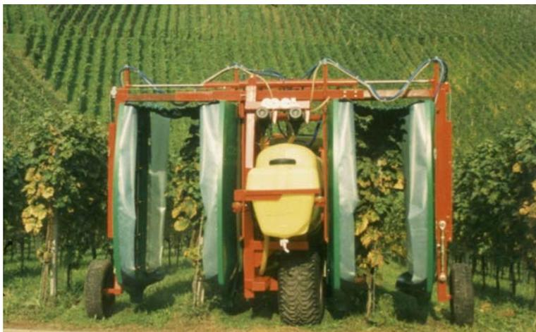
Fig. 3. Two-row tunnel sprayer in a vineyard.
