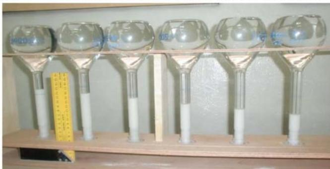
Fig. 7. Sedimentation tests made to determine the tracer concentration and the reference sedimentation time for each tracer examined.
