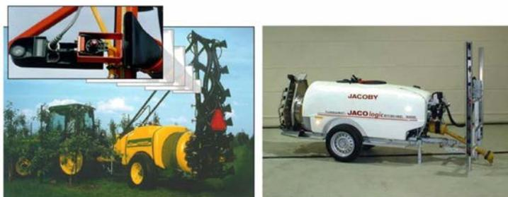
Fig. 2. Orchard sprayers with green detectors.
