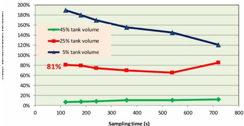
Fig. 14. Glass microspheres concentration in samples taken out of the 200 l tank when the agitation system was activated.
