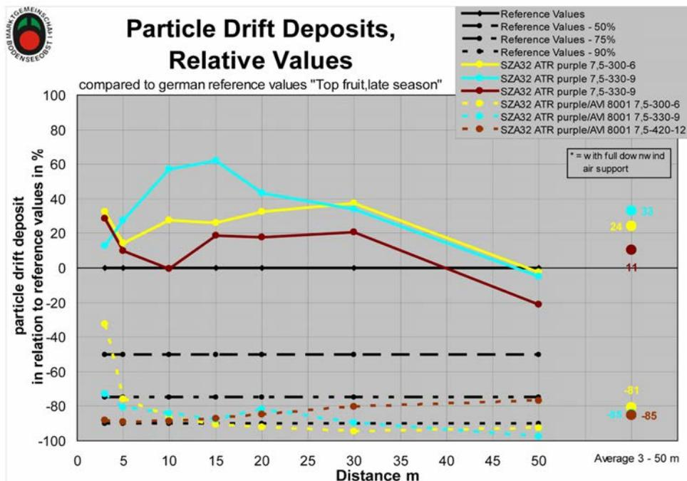
Graph 1. Particle drift deposits in relation to reference values "top fruit - late season" from a tower sprayer with canopy adapted fan speed at 6,0, 9,0 and 12,0 km h<sup>-1</sup>. Upper graphs: 16 x hollow cone nozzle "Albus ATR purple"; lower graphs: mixed nozzle set of 12 x hollow cone nozzle "Albus ATR purple" and 2 x AVI 8001.
