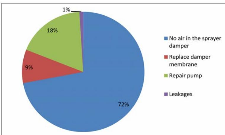
Fig. 11. Most common defects in pumps (MARTINS & NUNES, 2007).
