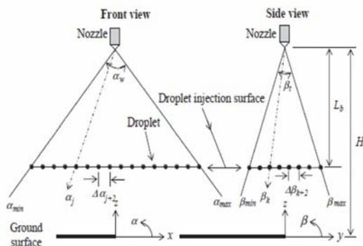
Fig. 1. Schematic showing the virtual nozzle with spray cloud boundaries, droplet injection surface, and droplet injection positions:  $x, y$  and  $z$ , coordinates;  $\alpha$  and  $\beta$  angular coordinates defining the spray boundary and droplet positions;  $H$ , nozzle height above the ground,  $L_b$  liquid sheet break-up length. [SIDAHMED and al., 2005].
