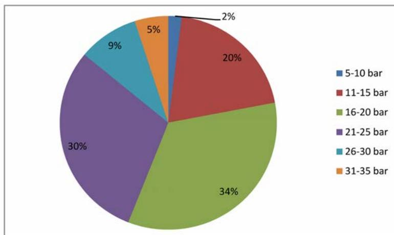
Fig. 5. Working pressures most used in orchard sprayers (MARTINS & NUNES, 2007).
