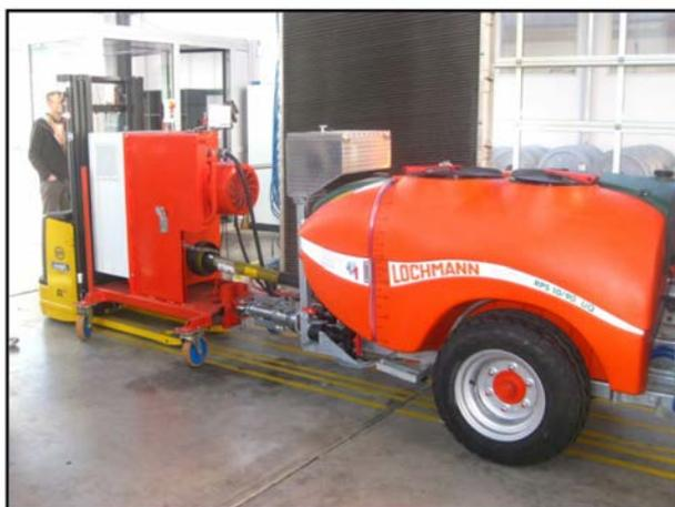
Fig. 2 Visit of the sprayer manufacturer Lochmann. Visit of the sprayer calibration facility and air-flow test stand.
