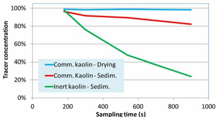
Fig. 10. Comparison between tracer concentrations measured in the tank samples after different sampling times, assessing the sedimentation levels in the flask necks or drying the samples in the heater.
