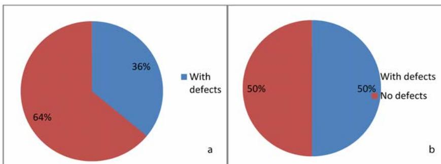
Fig. 9. Defects in pressure gauges of field crop sprayers (MARTINS & NUNES, 2007a), defects in pressure gauges of orchard sprayers (MARTINS & NUNES, 2007b).
