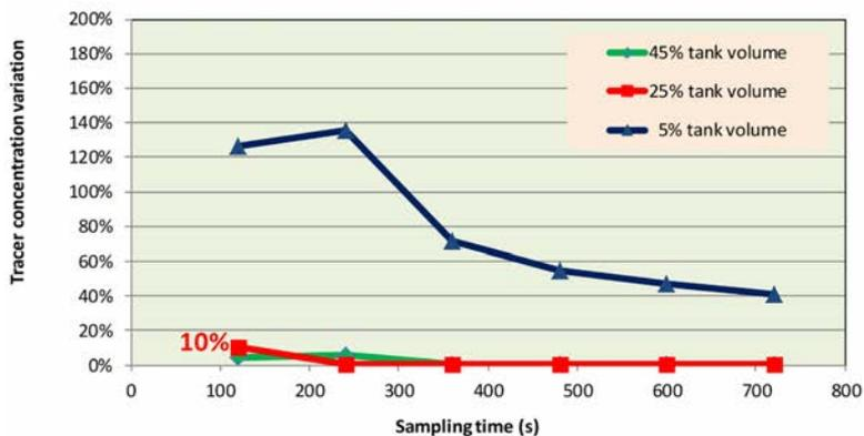
Fig. 13. Glass microspheres concentration in samples taken out of the 600 l tank when the agitation system was not activated.
