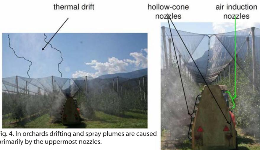
Fig. 4. In orchards drifting and spray plumes are caused primarily by the uppermost nozzles.
