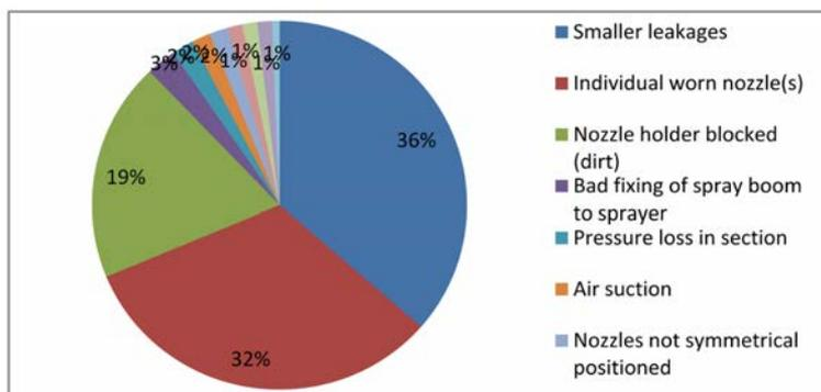
Fig. 6. An overview of category II defects during 2008-2009-2010 (Orchards sprayers).
