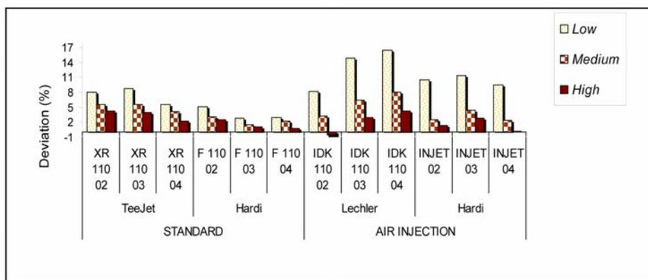
Fig. 3. Deviation values for the flow rate measured at three working pressures with an air-tight adaptor on different models of flat fan nozzles. The value of the pressure level (Low, Medium and High) is different for each nozzle model, so that it fits within its working pressure range.
