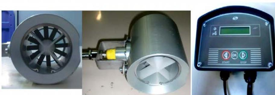
Fig. 4. Second type of sensor instrument equipped with an axial fan flow meter in a cylindrical body.
