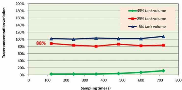
Fig. 12. Glass microspheres concentration in samples taken out of the 600 l tank when the agitation system was activated.
