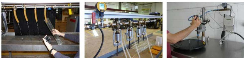
Fig. 2. Three methods for nozzle airflow measurement, graduated cylinder and stopwatch (left), air-tight nozzle adaptor (centre) and nozzle flow rate bench (right).
