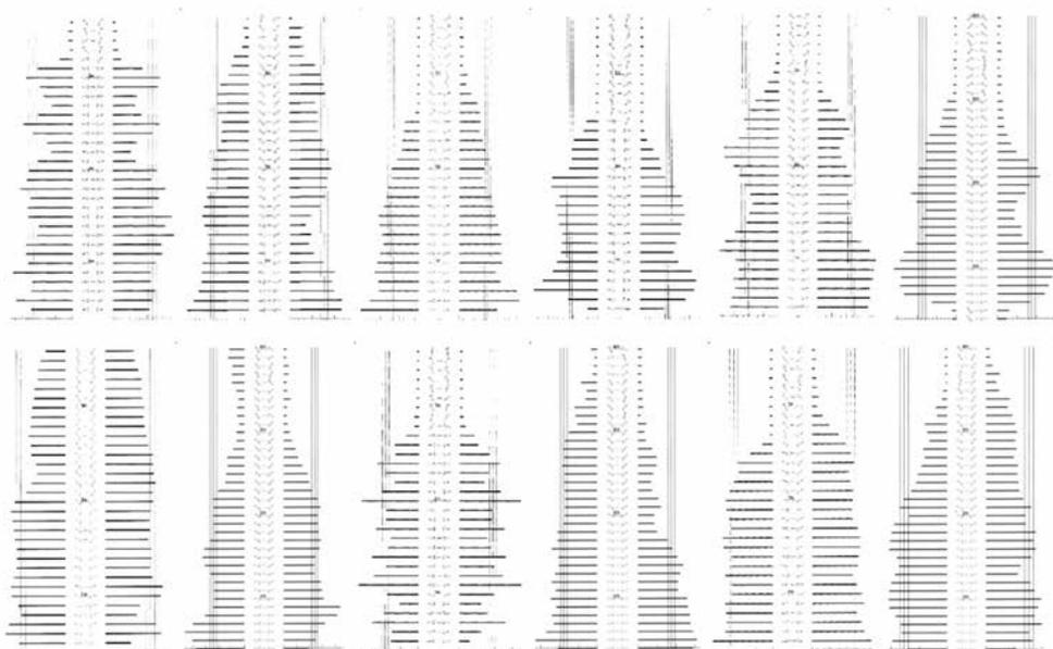
Fig. 3. Examples of the vertical air distribution of various types of fans of orchard sprayers with cross flow characteristics.
