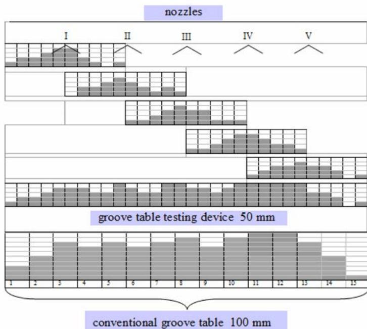
Fig. 4. Method of converting volumes of liquid table testing device (grooves 50 mm) for the table conventional patterner (grooves 100 mm)- virtual boom sprayer. Results of first tests and conclusion
