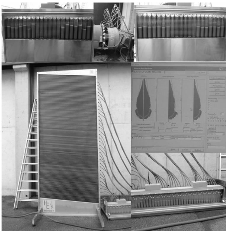
Fig. 3. Instrumental measurement of the nozzle flow rate and vertical distribution homogeneity during inspection and calibration activity.
