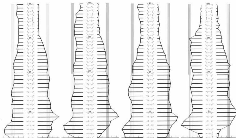
Fig. 4. One example of the varying vertical air distribution of individual fans from a series (axial fan with cross flow characteristics) for the treatment of tall trees (e.g. stone fruit).
