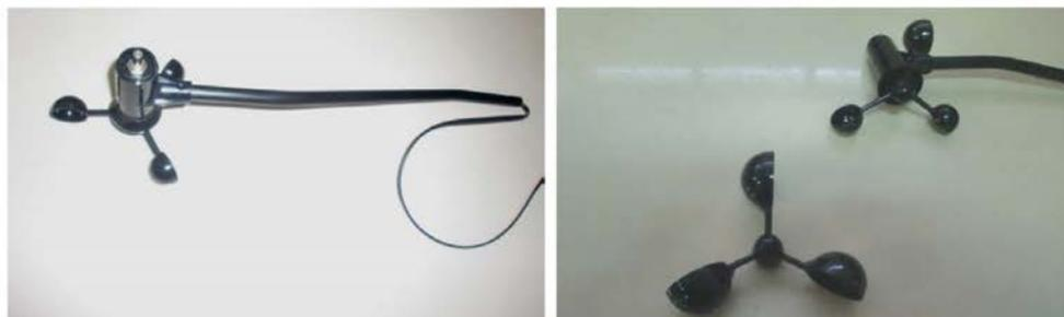
Fig. 5. Third type of sensor instrument, equipped with cup anemometer sensors.
