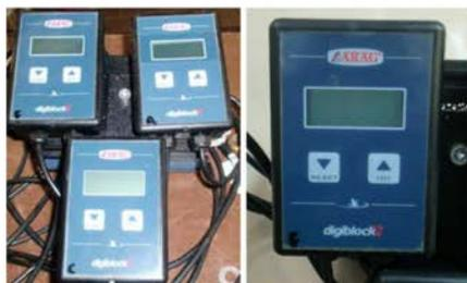
Fig. 3. Displays “Digiblock 2” manufactured by Arag company for visualization and registration of flowrate measurements.
