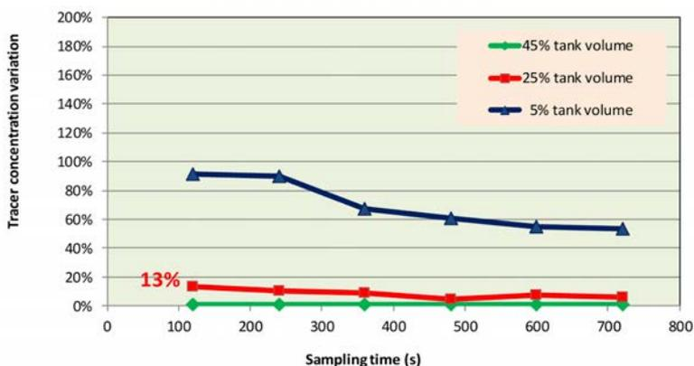
Fig. 15. Glass microspheres concentration in samples taken out of the 200 l tank when the agitation system was not activated.
