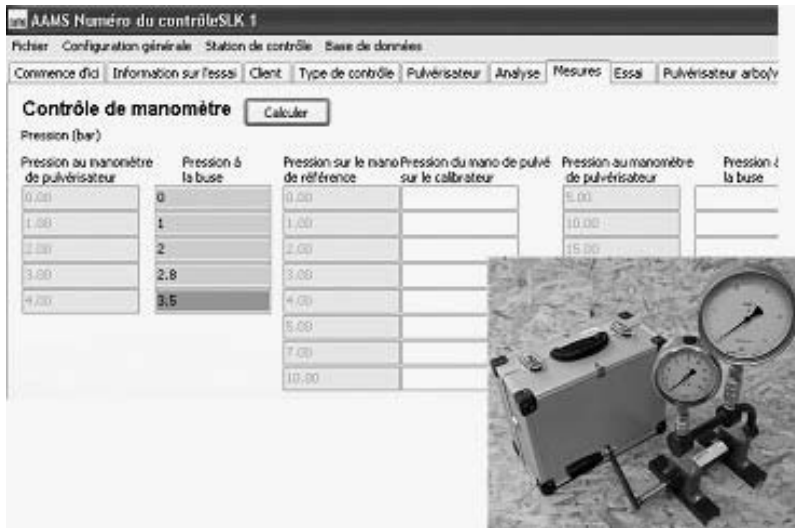
Fig. 1 Data of manometer verifications (up to 4 manometers, 8 different pressure levels possible for every individual manometer etc).
