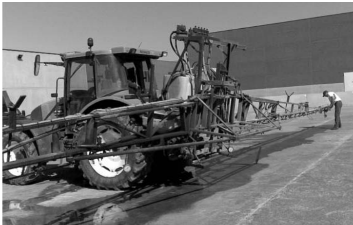
Fig. 1 Measuring pressure in different boom sections
