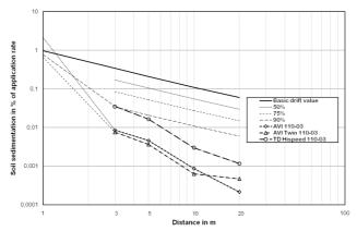
Fig. 2 Results of drift measurements.
