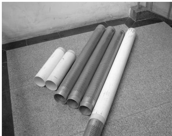
Figure 5 Solid and perforated piping components for one vertical aerator assembly.
