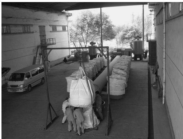
Figure 7 Flexible container attached to fan and duct assembly for drying.
