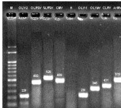
Fig. 1 Agarose gel electrophoresis analysis of amplified products obtained by one step RT-PCR using primers for the eight olive tree viruses (Table 1). Lane M, 100 bp DNA marker
