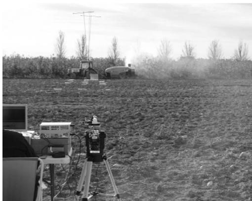
Fig. 1. Lidar system (foreground) measuring the spray drift generated by the sprayer (background).
