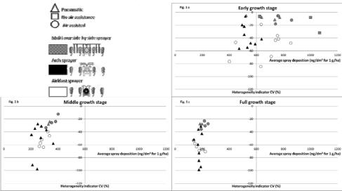
This synthetic representation enables to get a global view of vineyard sprayers' performance. The same scale has been voluntary used in the three graphics in order to view the effect of vegetation growth stage on deposits amount. At full growth stage, the gaps of performance between the different applications techniques are mainly linked to the homogeneity indicator whereas both indicators are showing differences of performance at early growth stage.
