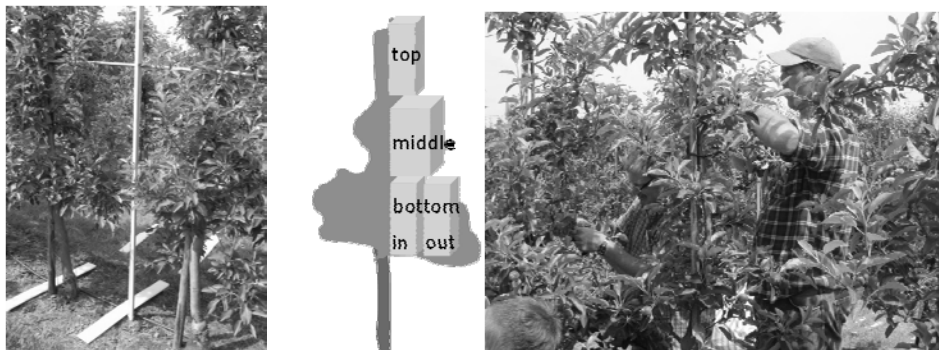
Figure 2. Spray deposition measurement on collectors on the ground (left), in the tree as leaf picking (right) following the sampling scheme (centre).
