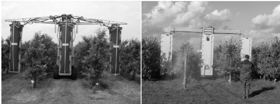
Figure 1. Munckhof 3-row sprayer (left) and KWH 3-row sprayer (right). Both sprayers were tested as 2-row sprayers spraying the tree rows alongside the sprayer from both sides.
