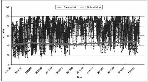
Figure 7 Relative humidity of the interstitial air and that of the ambient air over time of storage.
