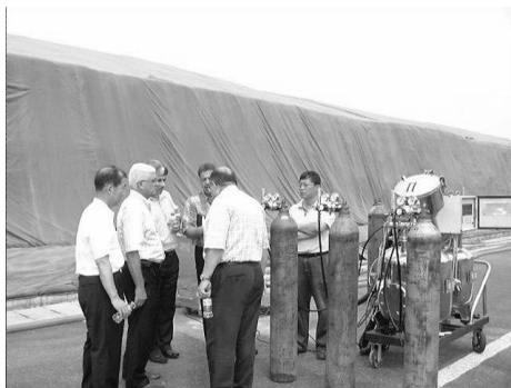
Figure 8 Phosphine recirculation fumigation system on big stack.
