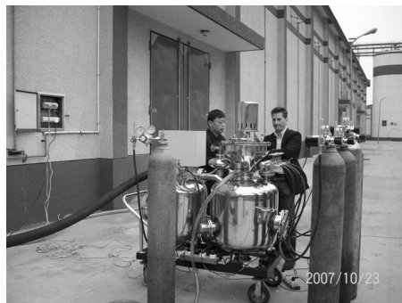
Figure 7 Phosphine recirculation fumigation system on big storehouse.
