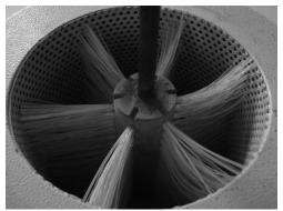
Figure 2 Inner view of pulse beetle egg removal device.
